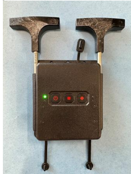
Figure 4: Probe charging position
